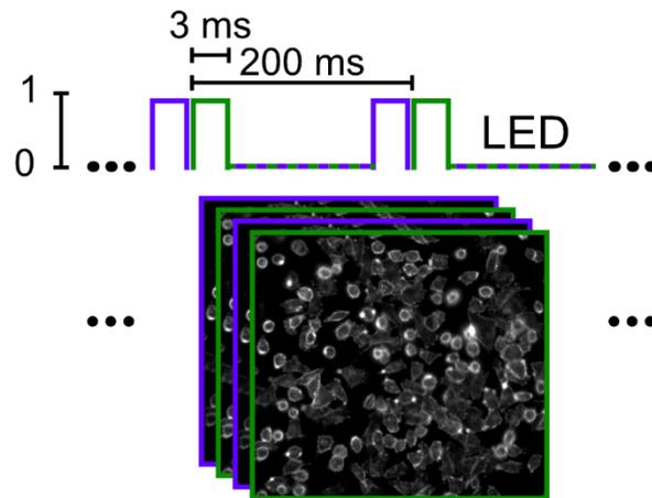
**Figure S1. Image acquisition timing diagram.** Top, illustration of the command signals sent to the LED illumination driver showing the length and duty cycle of the ratiometric illumination. Each color was sequentially strobed for 3 ms every 200 ms resulting in an interleaved series of fluorescent images (bottom).
