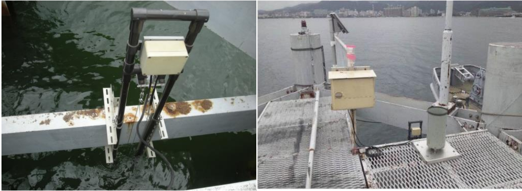
Fig. A3. Photos of the water level gauge (left) and observation site (right) with rain and water level gauges deployed at the Yanagasaki pier.
