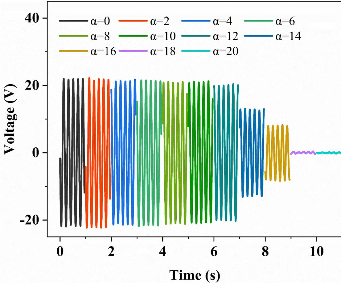
Figure. S9. Voltage variation of G-PENG with attack angle ( $\alpha$ ) at a wind speed of 6.24m/s, Related to Figure 2.
