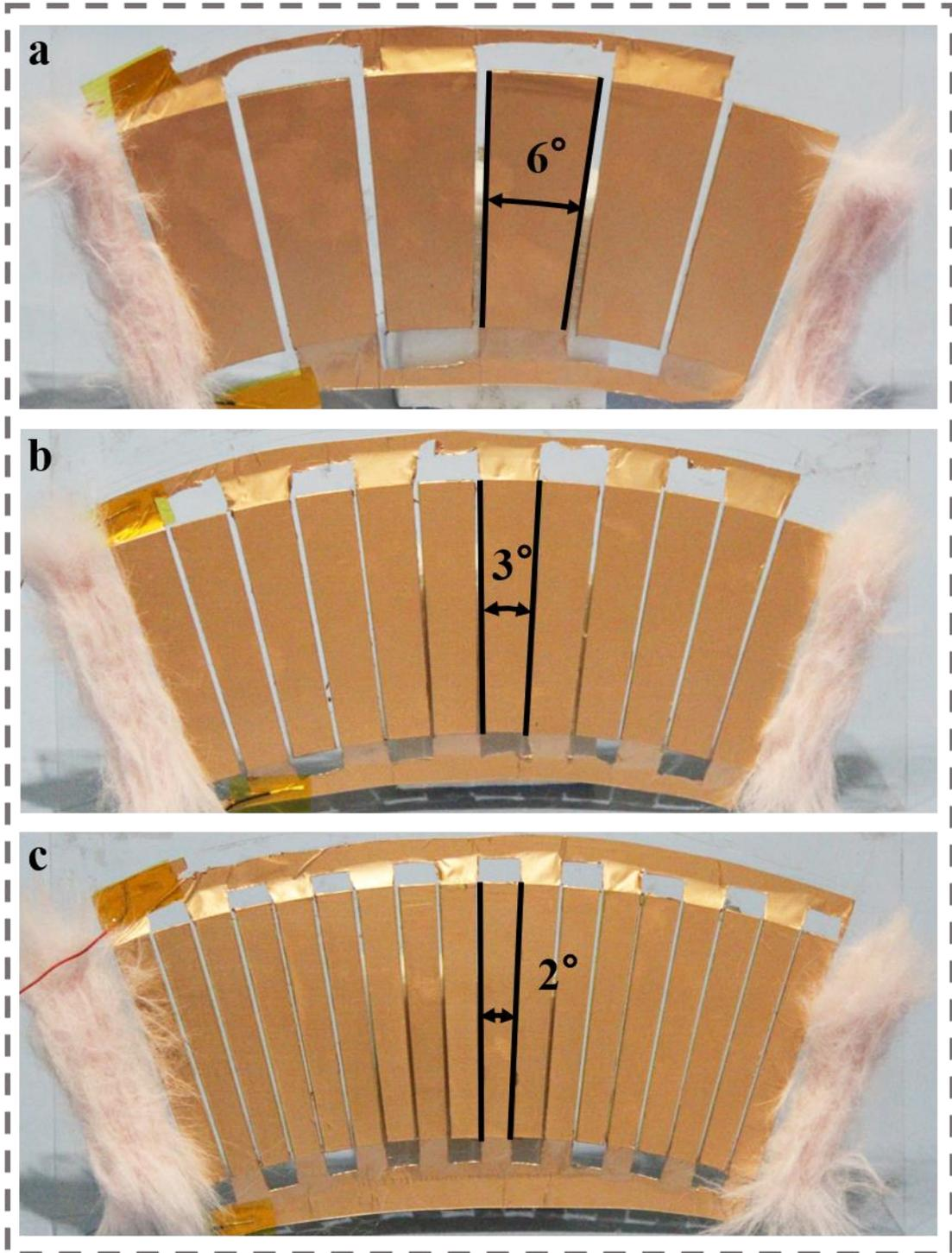
Figure. S5. Schematic diagram of the 3 types of electrodes: (a) 6-degrees, (b) 3-degrees, (c) 2-degrees G-TENG, Related to Figure 2.
