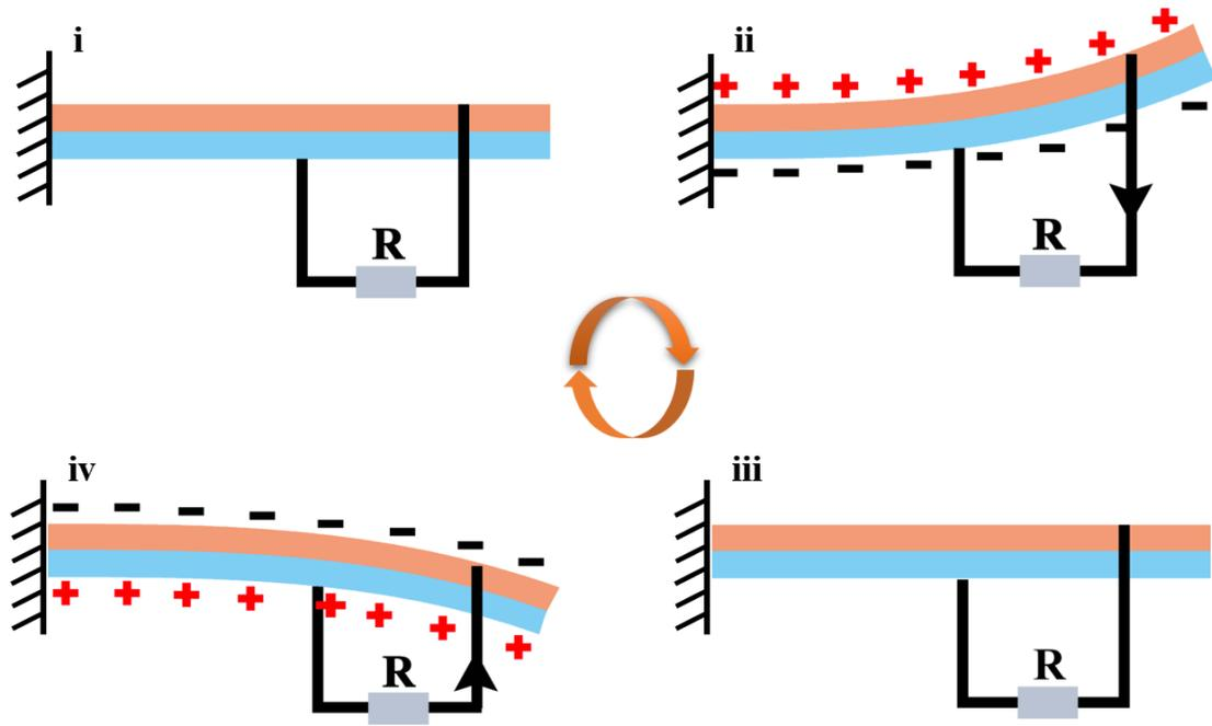
Figure. S2. Schematic diagram for the working principle of piezoelectric effect, Related to Figure 1.
