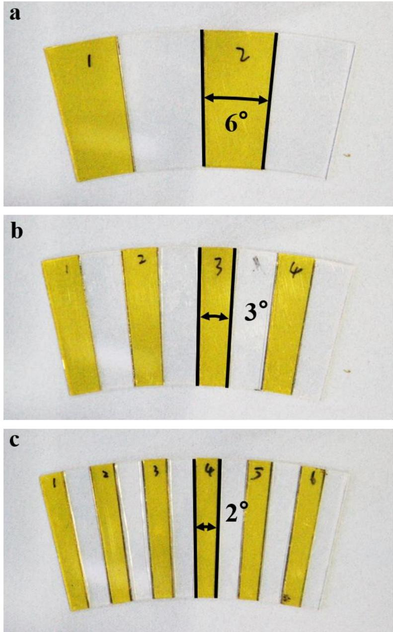
Figure. S1. Schematic diagram of acrylic plate with FEP (a) 6-degrees, (b) 3-degrees, (c) 2-degrees, Related to Figure 1.
