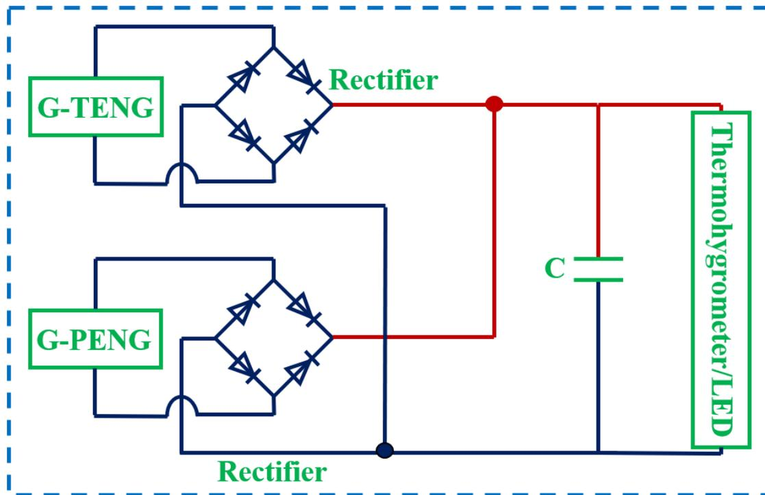
Figure. S10. Circuit diagram of HG P-TENG, Related to Figure 4.
