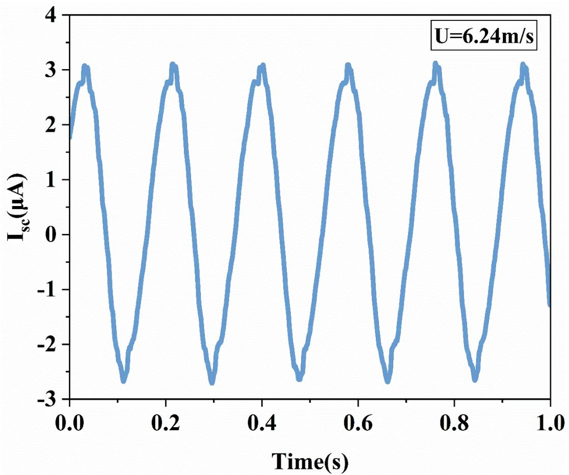
Figure.S7. Current of G-PENG at wind speed of 6.24m/s with resistance of  $9 \times 10^6 \Omega$ , Related to Figure 2.
