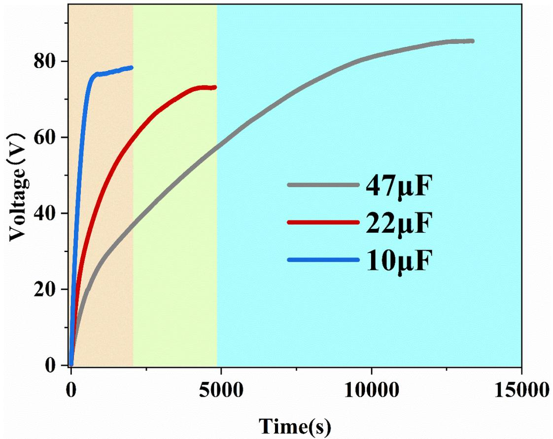
Figure. S11. Charging diagram of saturation voltage of various capacitors (3-degrees), Related to Figure 3.
