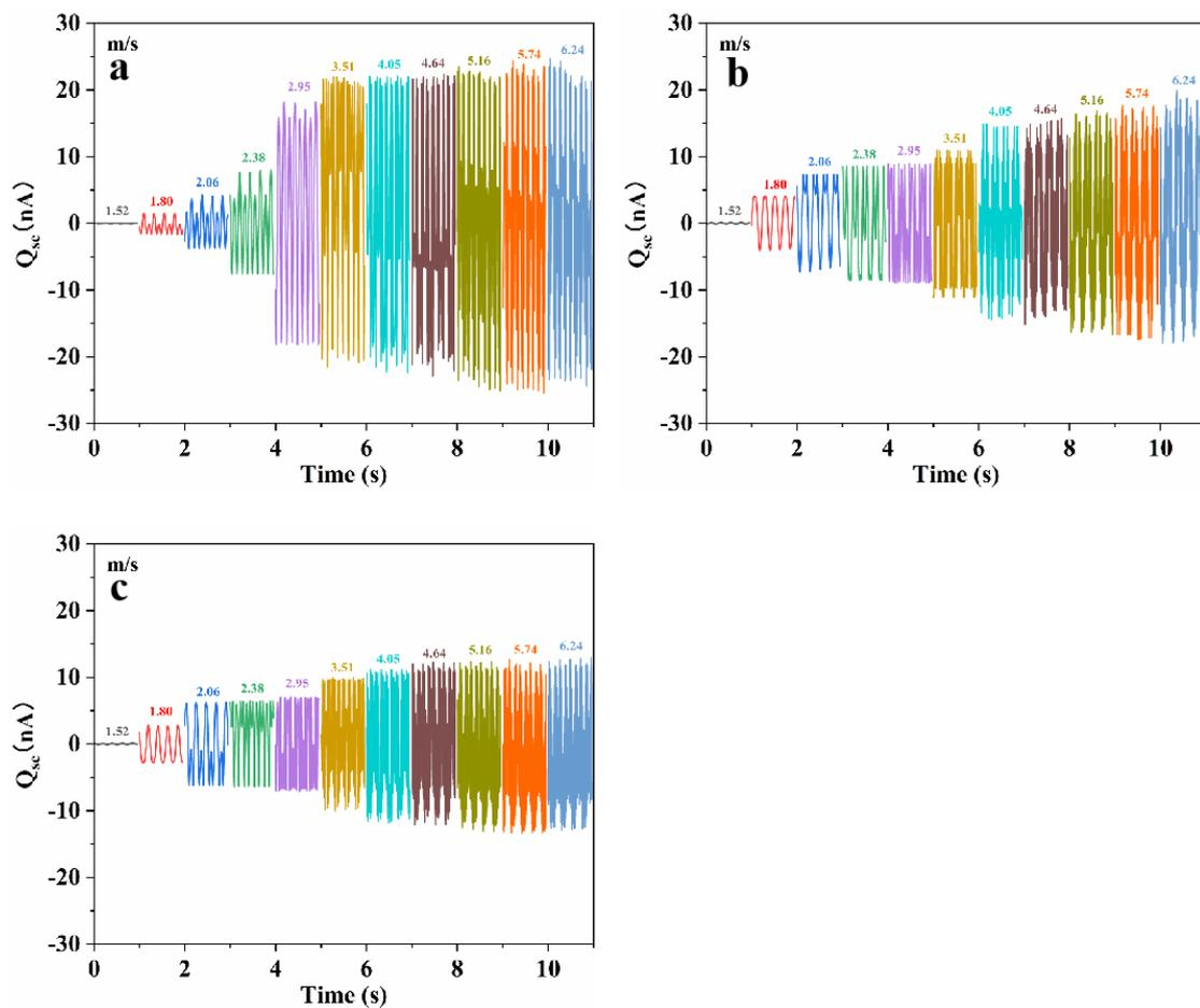
Figure. S3. Transfer charge of (a) 6-degrees, (b) 3-degrees and (c) 2-degrees G-TENG,
