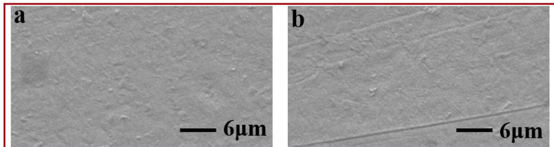
Figure.S14. Comparison of SEM images of FEP material (a) before and (b) after friction, Related to Figure 1.
