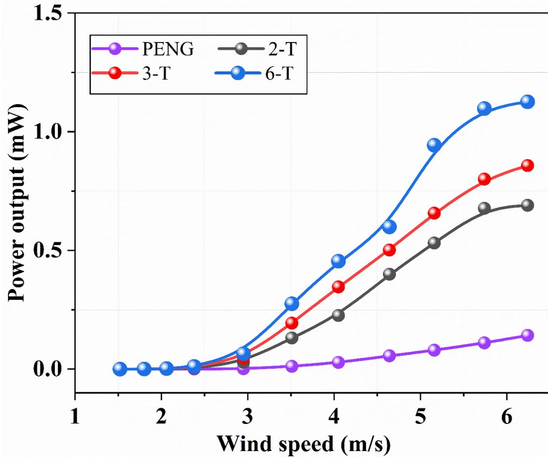
Figure.S13. The peak power of 6-degrees, 3-degrees, 2-degrees G-TENG and G-PENG variation with wind speed, Related to Figure 4.
