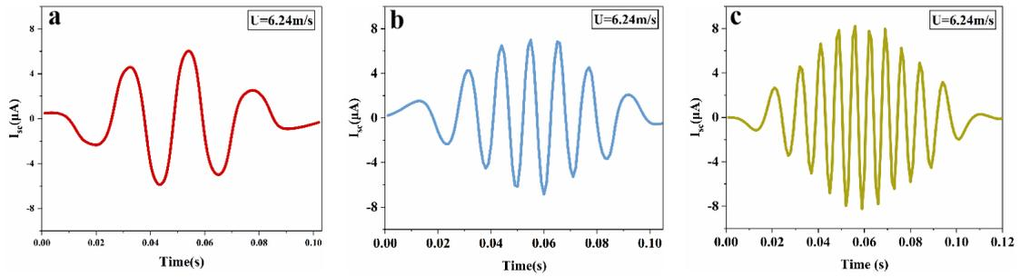
Figure.S6. Current scale-up for (a)6-degrees, (b)3-degrees, and (c)2-degrees G-TENG at wind speed of 6.24m/s, Related to Figure 2.
