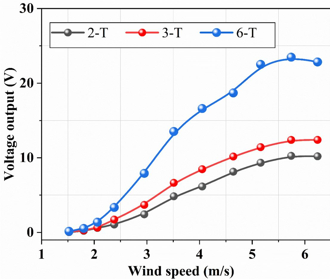
Figure.S12. RMS voltage of the 6-degrees, 3-degrees, 2-degrees G-TENG variation with wind speed, Related to Figure 4.
