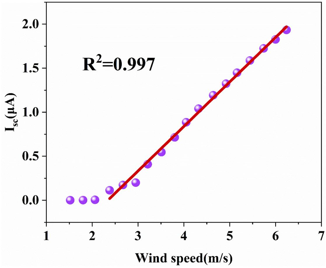
Figure.S8. Variation of the RMS current of G-PENG with wind speed, Related to Figure 2.
