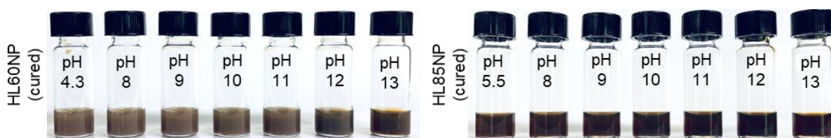
Figure S4. Stability of cured HLNPs in alkaline aqueous solutions at different pH.
