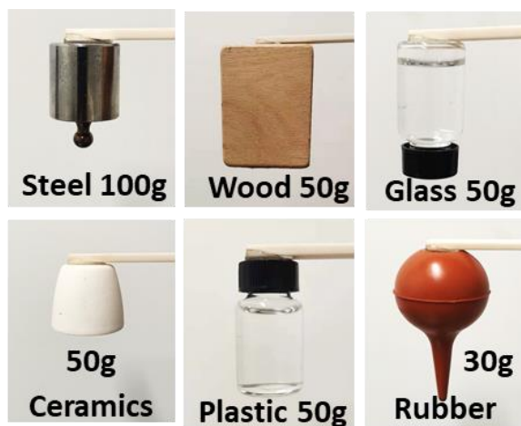
Figure S3 Photographs of the poly(PBA- ran -PDMS) adhering to various substrates: steel, wood, glass, ceramics, plastic and rubber.
