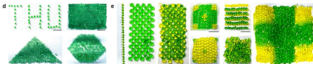
Figure R34. (left) Homogenous structures of printed gelatin beads, including a THU alphabetical sparse pattern, and rectangular, triangular and hexagonal dense patterns. (right) Heterogeneous structures of printed gelatin beads of two different colours. Scale bar, 5 mm.
