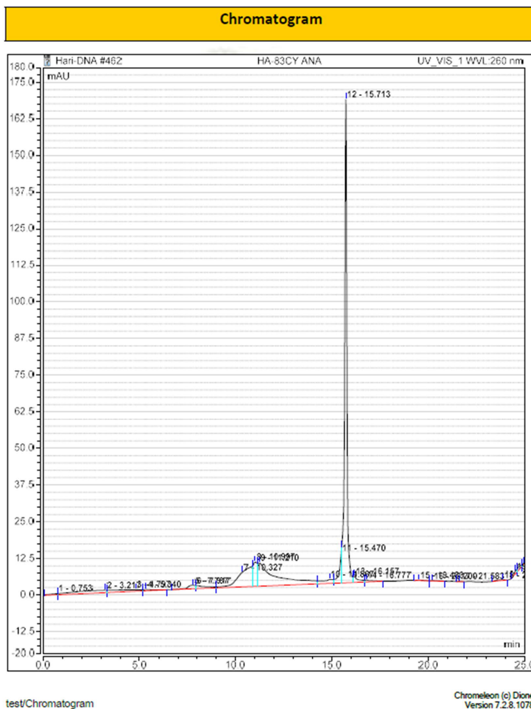
Figure S75. Reverse phase HPLC profile of dZ[U E (-3), A N3 (+1)]X. Note that the broad peak at 11 min is an artefact of the column.
