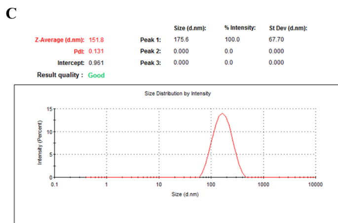
Figure S2. Dynamic light scattering data of bare cubosomes (A), CuAc-loaded cubosomes (B) and CuAc-loaded, HA-tagged cubosomes (C).
