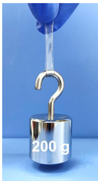
Fig. S3 Photographs of the stretching behavior for CTA hydrogel under a weight loading of 200
