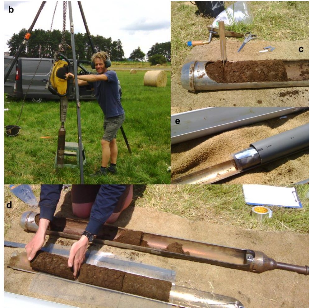
8 9 Supplementary Fig. 2. Soil core sampling and microcosm preparation method. A percussion core drill equipped with a steel tube that can be 10 opened from sideways was used to extract intact soil columns of 8 cm diameter ( a , b , d ). For each layer, three soil cores collected with a knife ( c ) 11 from the same depth in the initial soil column were gently stacked together ( a , d ), tightly sealed within a polyethylene sheath ( d , e ) and transferred 12 into a bottom-capped polyvinyl chloride (PVC) tube ( e ) to form a new soil column exclusively made of topsoil or subsoil ( a ). See Supplementary 13 Fig. 5 for the soil core sampling design of each soil type.
