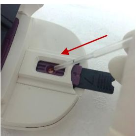
18. Apply mixed specimen to the specimen application hole of the test device
