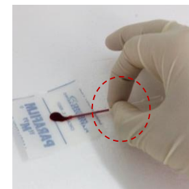
13. Hold the EZI tube horizontally, and touch the tip of the EZI tube to the blood specimen. Do not close hole.
