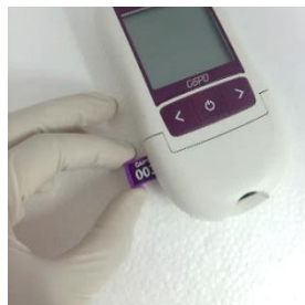
2. Insert codechip (For first time using or open new box of test device)
