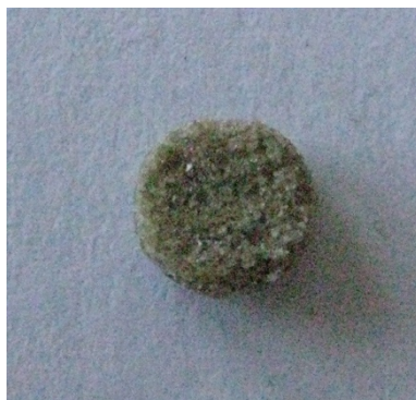
Supplementary Figure 35. Photograph of a_g ZIF-62 obtained after the preparative TGS/DSC experiment.
