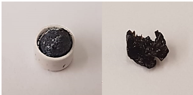
Supplementary Figure 33. Photographs of a_g ZIF-4 obtained after the preparative TGS/DSC experiment.
