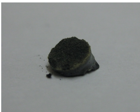
Supplementary Figure 34. Photograph of a_g ZIF-zni obtained after the preparative TGS/DSC experiment.
