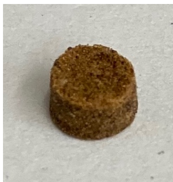
Supplementary Figure 36. Photograph of a_g TIF-4 obtained after the preparative TGA/DSC experiment.
