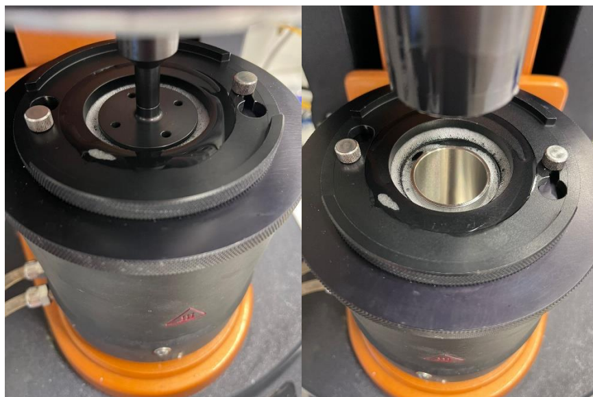
Figure S10. Foam formation for hydrophobically modified polymers during DR experiments in the rheometer.
