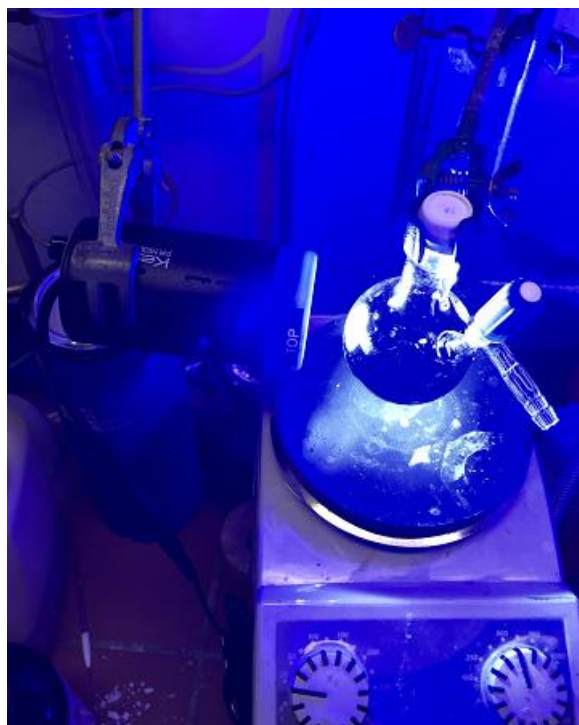
Supplementary Figure 2. Batch reactor set-up with light irradiation
