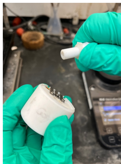
Left: Solution of nickel, ligand, RAE and arene after stirring for 10 minutes. Center: (optional) removal of the screwcap on the Electrasyn 2.0 Right: (optional) removed screwcap on the Electrasyn 2.0 vial.
