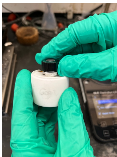
Left: Solution of nickel, ligand, RAE and arene after stirring for 10 minutes. Center: (optional) removal of the screwcap on the Electrasyn 2.0 Right: (optional) removed screwcap on the Electrasyn 2.0 vial.
