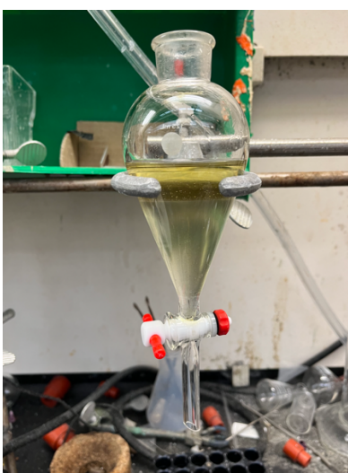
Left: Reaction mixture upon completion. Center: Crude reaction mixture partitioned between ethyl acetate in sat'd sodium bicarbonate. Right: Combined organic fractions dried over magnesium sulfate.
