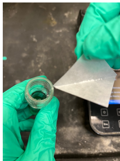
Left: Select “No” when prompted about alternating polarity. Center: Select “No” when asked to save experiment. Right: Addition of silver nitrate to the homogenous reaction solution.
