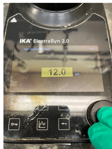
Left: Select “New Experiments”. Center: Select “Constant Current”. Right: Set the current to 12 mA
