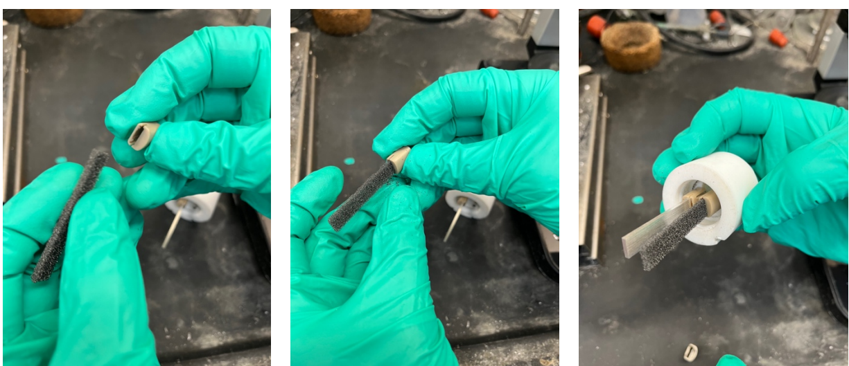
Left: Assembly of the RVC electrode. Center: Insertion RVC electrode into the beige clip. Right: Attached RVC electrode on the right of the cap.
