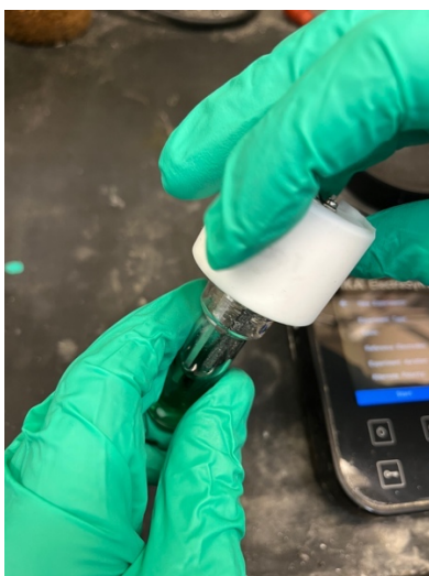
Left: Attachment of the cap to the Electrasyn 2.0 vial. Center: Attached vial to the Electrasyn 2.0. Right: Start of the reaction.
