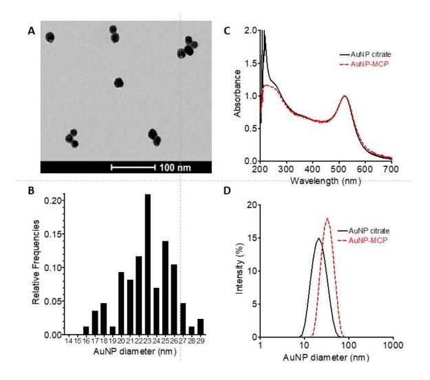
**Figure S2.** (A) TEM images of synthesized AuNPs. (B) Size distribution measured by TEM. (C) UV-visible spectra of AuNPs and AuNPs conjugated to MCP. (D) Size distribution of AuNPs and MCP-conjugated AuNPs measured by DLS.
