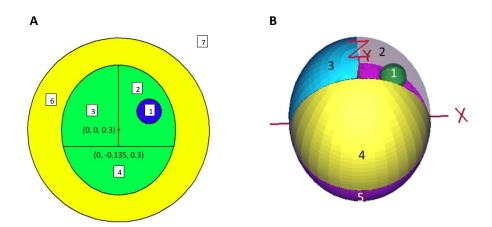
**Figure S1**. Schematic geometry used in the MCNP simulation. (A) x-y plane through the center (0.25, 0.15, 0.30 cm) of a 0.2 cm diameter tumor sphere (blue, labeled 1) in the mouse brain (green) enclosed by a 1.6 cm diameter spherical buffer (yellow, labeled 6) representing the mouse head,
