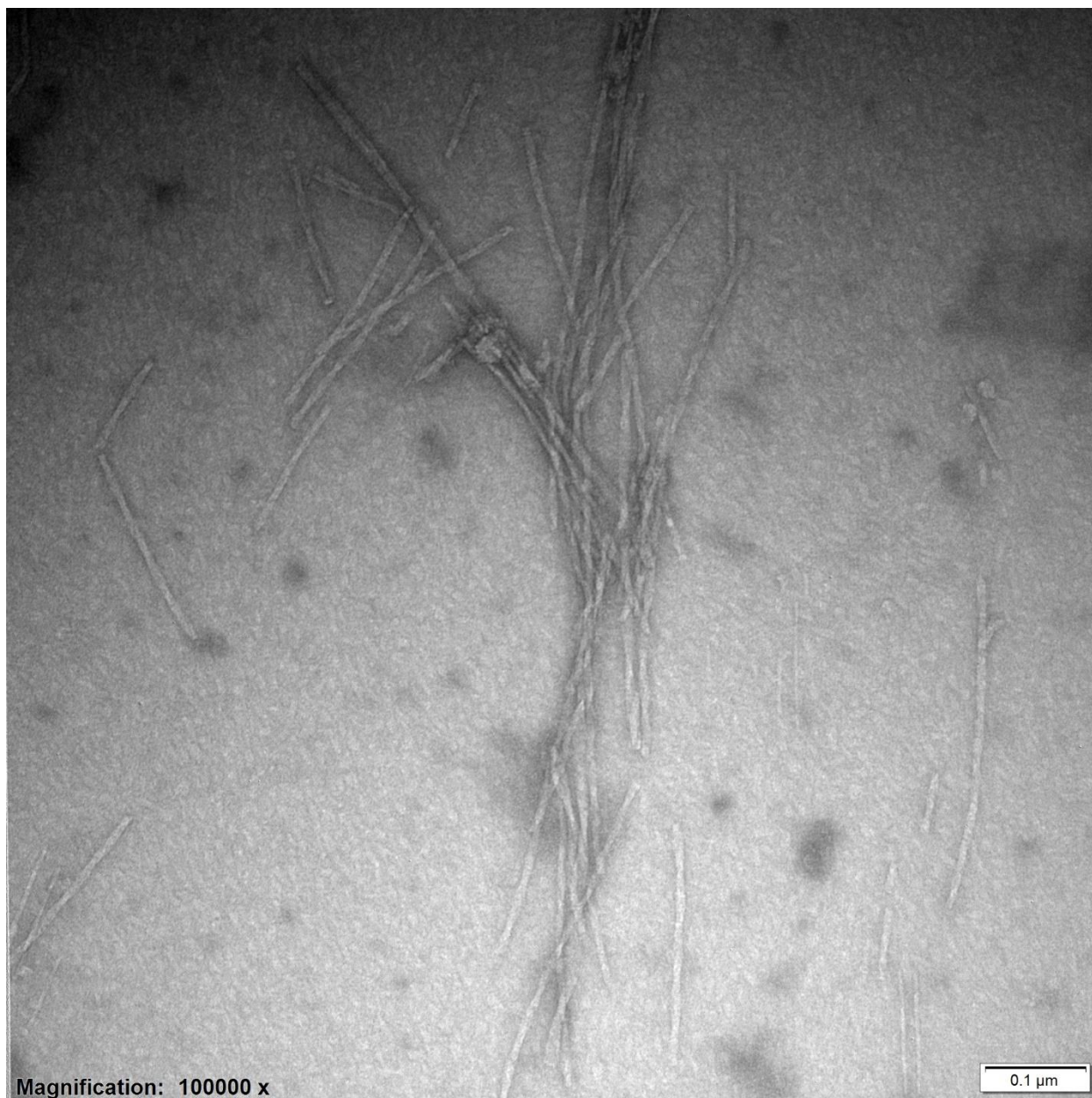
Supplementary Fig. 2: TEM micrograph of Q11 nanofibers.
