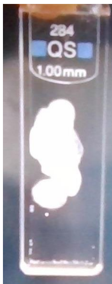
Figure S2: Picture of 1 mm cuvette with precipitated polymer after irradiation of a solution of 6.73 \text{ mol L}^{-1} DMA, 9 \text{ mmol L}^{-1} AIBN and 50 \text{ }\mu\text{L} AuNR.
