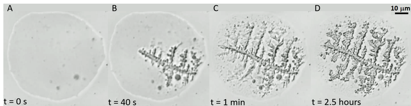
Fig. S6. Time series of microscope images (50x) of an efflorescing synthetic lung fluid (SLF) particle deposited on a hydrophobically coated substrate in a temperature and humidity controlled cell. The setup is described in detail by Ciobanu et al. (52). At 20.5°C and 54% relative humidity the particle's radius is approximately 40 \mu\text{m} (scalebar represents 10 \mu\text{m} ). (A) Liquid particle at t = 0 , when efflorescence begins. (B) 40 s after the start of crystallization with rapid dendritic NaCl crystal growth. (C) 1 min after initial crystallization the crystal reaches the edge of the droplet, slowing the speed of further crystallization dramatically. (D) 2.5 h after initial crystallization the crystal is still growing slowly, leading to a coarsening of the crystal structure. The size of the dendrites is used to calculate the morphology-dependent effective diffusion constant of \text{Na}^+ and \text{Cl}^- ions in the remaining, mainly organic solution (see section "Boundary condition at the liquid-solid interface and dendritic crystal growth habit").
