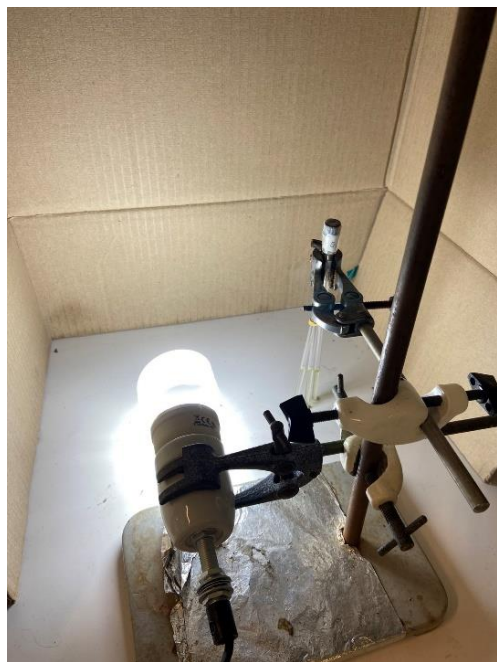
Figure S4. Set-up of photo-isomerization with white/UV light
