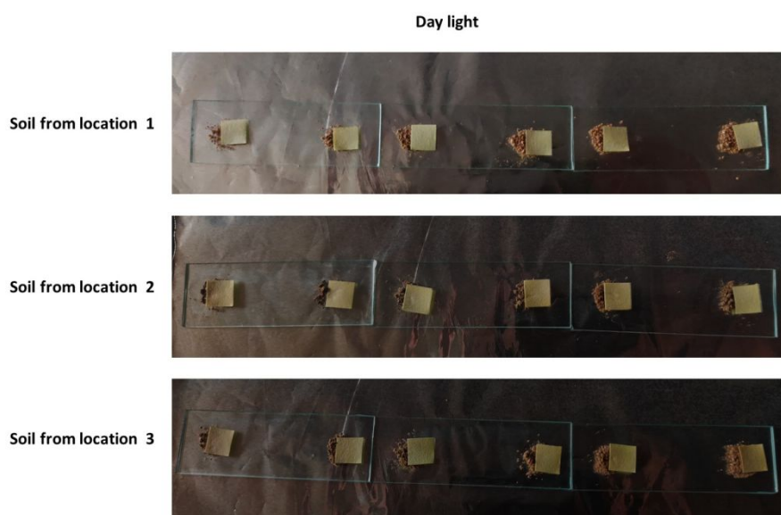
Figure S25. Photographs of portable paper strips under day light while contacting with soil samples already spiked with different concentration of TNT.
