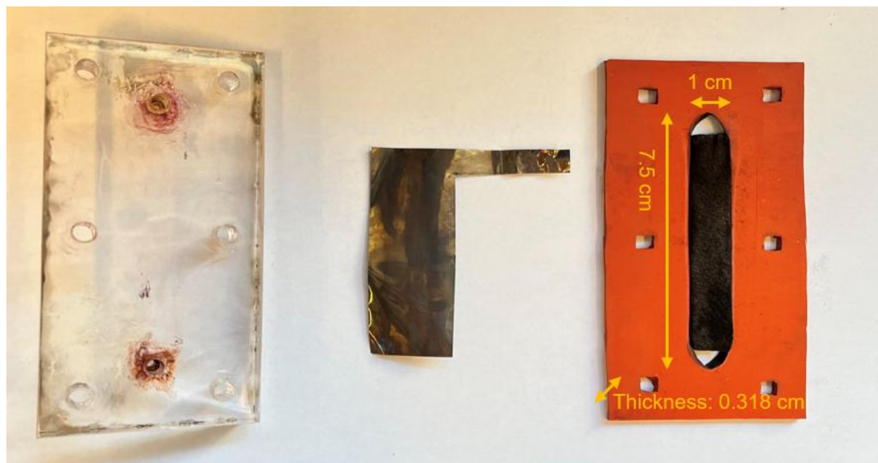
Supplementary Figure 8. Photograph of the flow cell.
