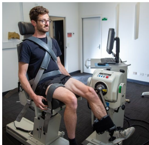
Figure SF3.3 Set up of knee muscle strength assessment using Biodex isokinetic dynamometer
