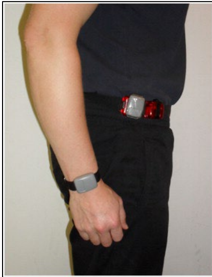
Example of accelerometer placement
