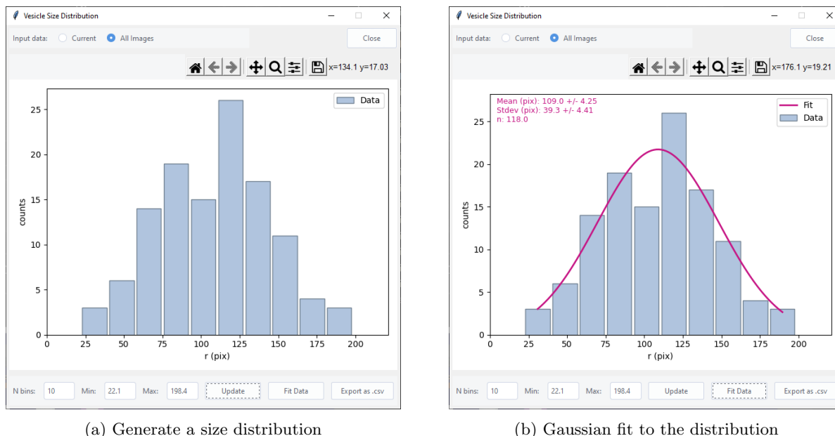
Figure 19: Size distributions. After vesicle detection, size distributions can be generated from the current image or all analysed images (a). The distribution can be fitted with a Gaussian and the results can be exported (b).
