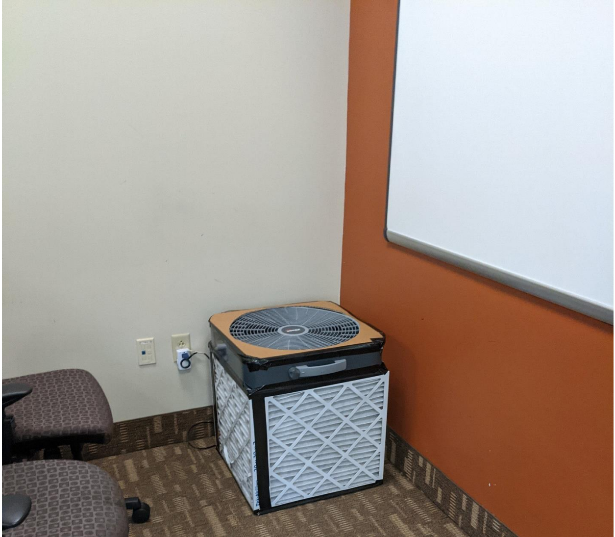
Supplemental Figure 1: Representative image of an assembled Corsi-Rosenthal box used in the intervention study.
