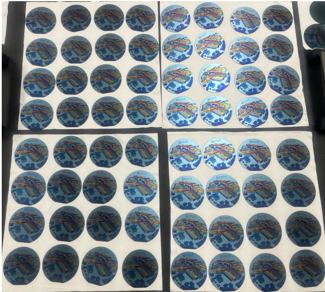
Supplementary Fig. 9 Repeatability tests. Photograph of 64 identical samples that are printed with the same laser parameters.
