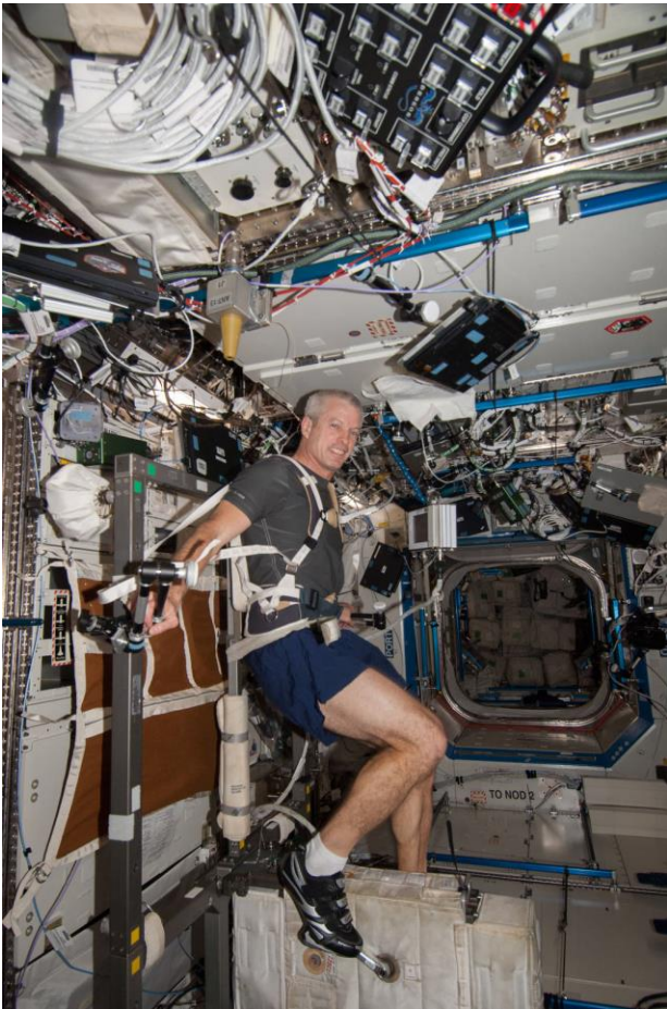
Supplemental Figure 2. Cycle Ergometer with Vibration Isolation System (CEVIS) on ISS. NASA Image: SS039-E-014696; https://www.nasa.gov/multimedia/guidelines/index.html
