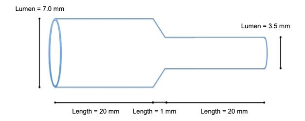
**Supplementary Figure 1.** Parameters of the bench vessel models.
