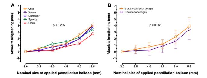
**Supplementary Figure 3.** Lengthening according to different stent types (A) and according to different type of stent designs (B).
