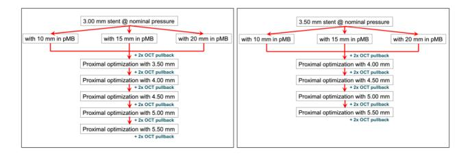
**Supplementary Figure 2.** Steps of the bench testing for the 3.00 mm stent platform (left) and for the 3.50 mm stent platform (right).
