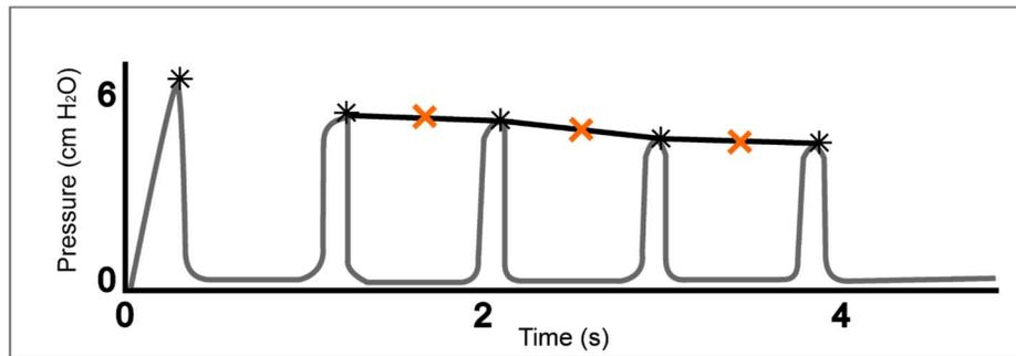
**Figure S2.** Estimation of the subglottic pressure from the intraoral pressure oral signal. Intraoral pressure for five /pae/ syllables showing peak values as orange asterisks and interpolation lines indicating estimated subglottal pressure halfway between peaks. Adapted from Espinoza et al. (2017).
