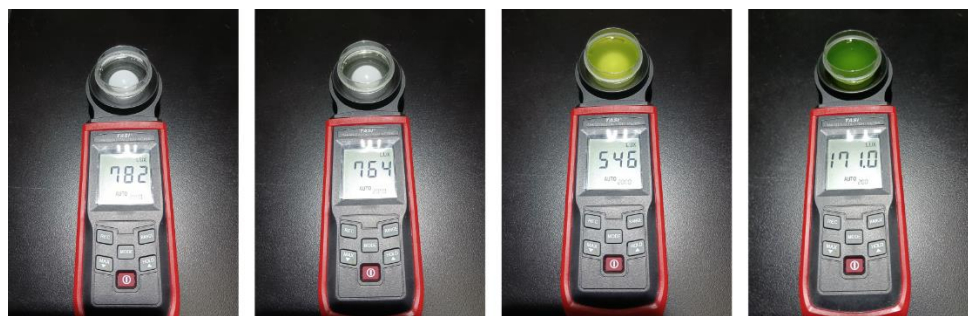
Figure S4 Light intensity attenuation by Chlorella hydrogels, left to right: CH6, CH7, CH8 and CH9.
