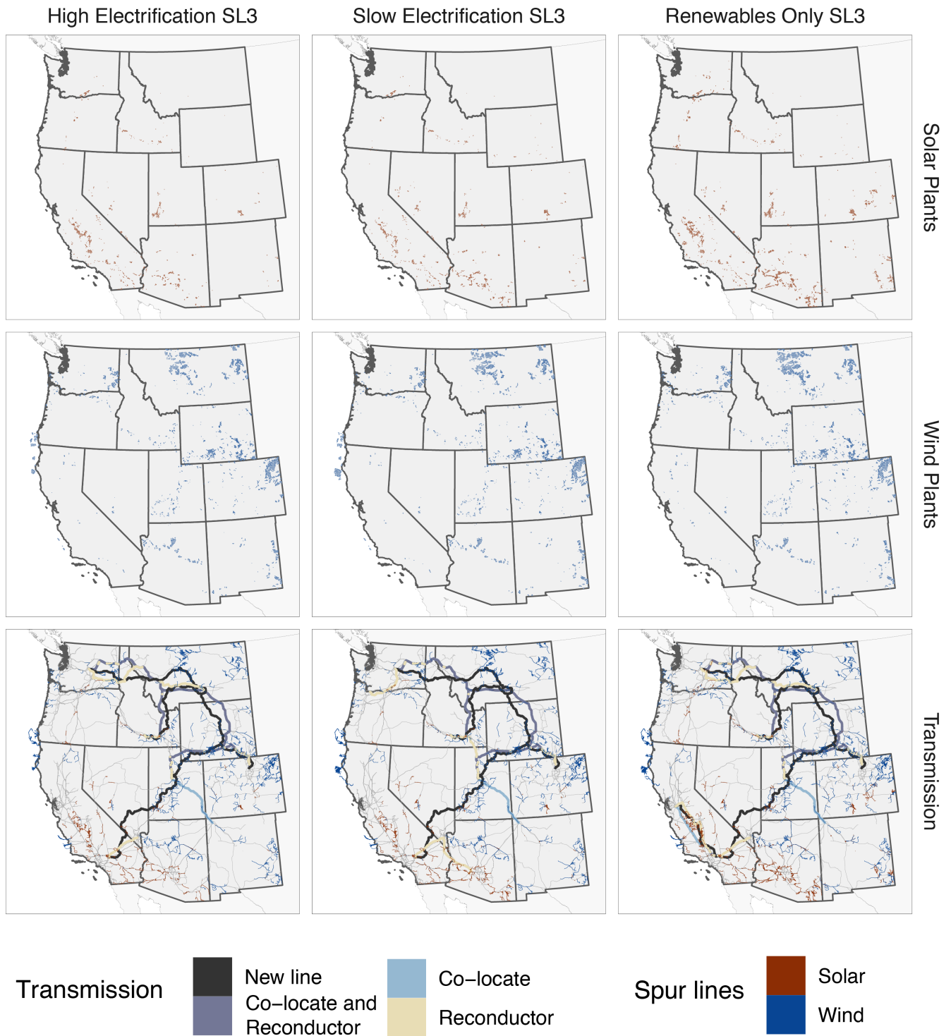
Fig. S24. Wind, solar, and power line build-out maps for Siting Level 3 of three main decarbonization cases (High Electrification, Slow Electrification, Renewables Only)
