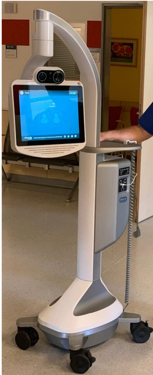
Figure S1. Photograph of the tele-ICU equipment to remotely monitor off-site ICU patients (intensive care telemedicine service provided by the tele-ICU cockpit located at Charité): Tele-medical cart with three cameras, directional microphone, power cord shelf hook, privacy handset, shelf, handle, expansion bay, power plug and cord, wheel locks and a basket.
