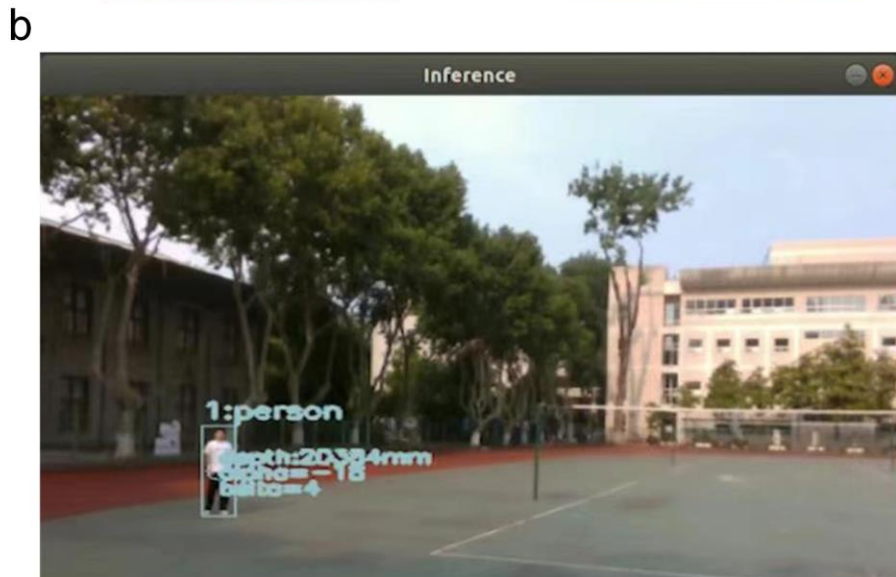
Supplementary Fig. 1 (a) Mapping diagram of pixel plane and reality plane, captured range of the RS-camera based on the geometrical optics. (b) The actual measured scene displayed on the computer. Outdoor performance of the RS-Camera, when the target is about 20m away from the RS-Camera.
