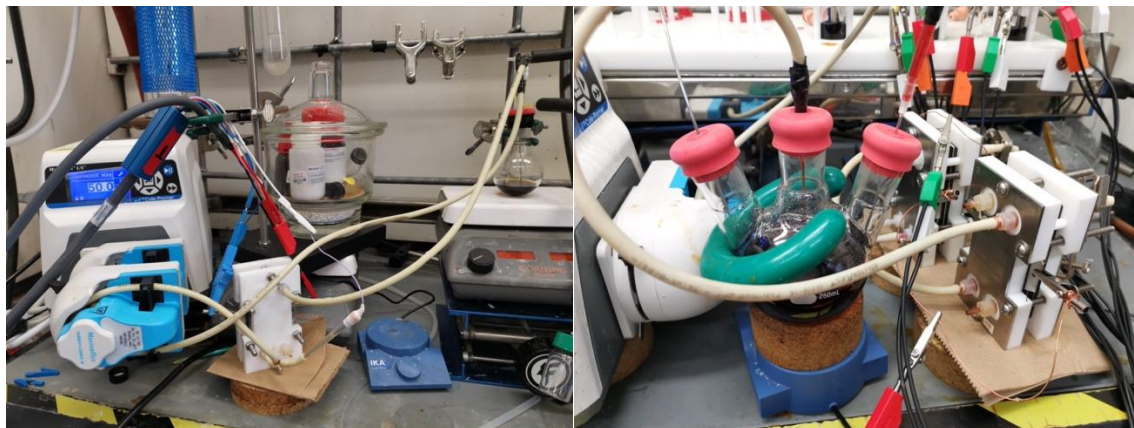
Figure S4. Graphic illustration of the undivided flow cell for 12 mmol (left) and 48 mmol (right) scale-up.
