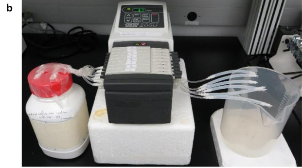
Supplementary Figure S3. Characterization of catheter-biofilm formation in a continuous flow model. (a) Experimental timeline of the biofilm formation test. (b) Schematic diagram of continuous flow catheter system, including influent, peristaltic pump, urinary catheter, and effluent. AUM: artificial urine medium (AUM).
