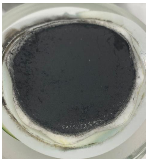
Figure S1. Digital photo of borophene depositing on the surface of cellulose paper. External forces like scratching and folding could easily wipe out the borophene powder.
