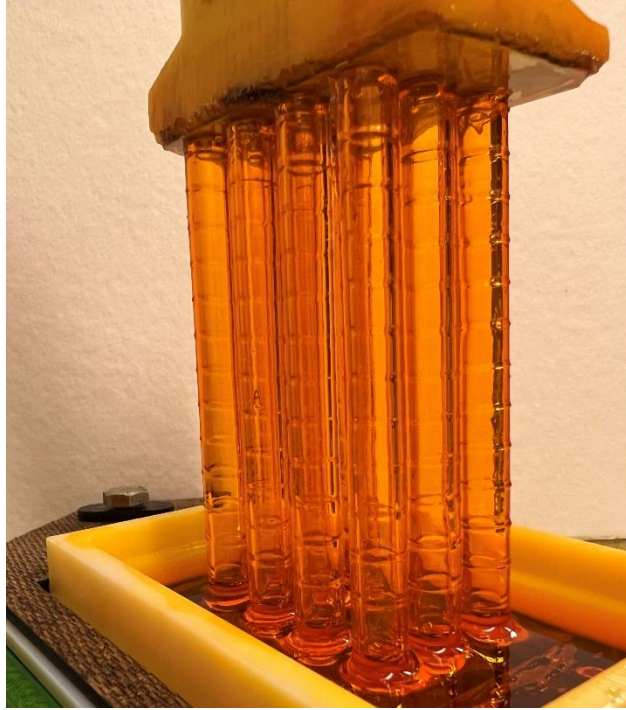
Figure 22. Photo of a g-DLP printing of 12 tentacle-like actuators in one batch, printing speed 1mm/min.
