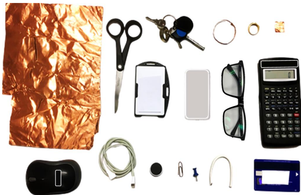
Figure S2. The magnetic objects tested during the fluctuation tests of the EMT systems.
