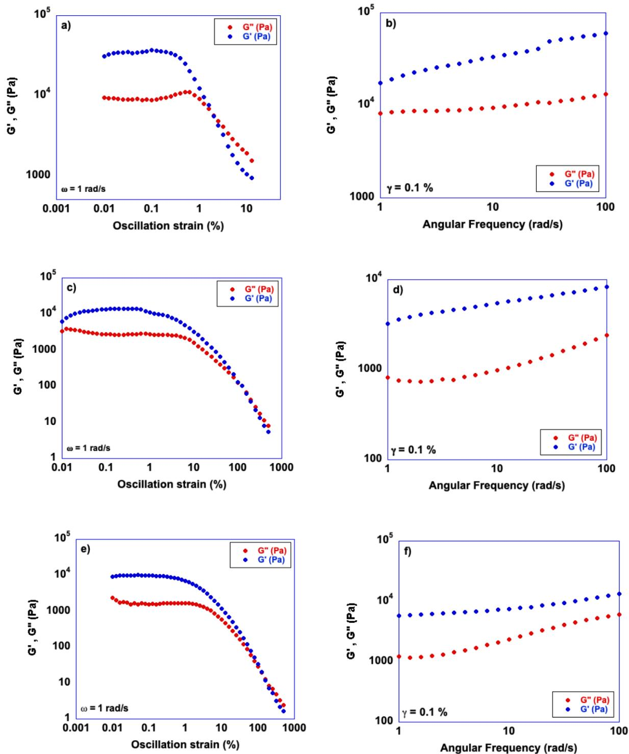
**Figure S1.** Strain- and frequency sweeps of 3 wt% gels in a), b), [bmpip][NTf<sub>2</sub>]; c), d), [bmim][PF<sub>6</sub>]; e), f), [bmim][NTf<sub>2</sub>];
