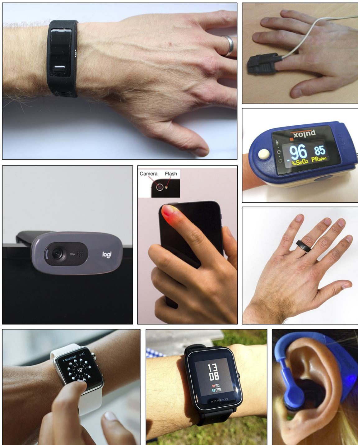
Figure 1. Devices for measuring the photoplethysmogram (PPG) signal. The PPG can be measured by several clinical and consumer devices, including (clockwise from top left ) wristbands, pulse oximeters ( \times 2 ), smart rings, smartwatches, hearables, smartwatches ( \times 2 ), webcams, and smartphones. Sources (clockwise from top): P. H. Charlton, Max Health Band ( https://commons.wikimedia.org/wiki/File:Max_Health_Band.jpg ) ( https://creativecommons.org/licenses/by/4.0/ CC BY 4.0); P. H. Charlton, Wrist pulse oximeter ( https://commons.wikimedia.org/wiki/File:Wrist_pulse_oximeter.jpg ) ( https://creativecommons.org/licenses/by/4.0/ CC BY 4.0); Stefan Bellini, Pulox Pulse Oximeter.JPG ( https://commons.wikimedia.org/wiki/File:Pulox_Pulse_Oximeter.JPG ) ( https://creativecommons.org/publicdomain/zero/1.0/ CC0 1.0) M. Verch, https://flickr.com/photos/160866001@N07/32586534637/ ( https://creativecommons.org/licenses/by/2.0/ CC BY 2.0); S. Passler et al. (242) https://doi.org/10.3390/s19173641 ( https://creativecommons.org/licenses/by/4.0/ CC BY 4.0); GEEK KAZU, https://www.flickr.com/photos/152342724@N04/36729615770/ ( https://creativecommons.org/licenses/by/2.0/ CC BY 2.0); L. Chesser, Apple_Watch_user_(Unsplash) ( https://commons.wikimedia.org/wiki/File:Apple_Watch_user_(Unsplash).jpg ) ( https://creativecommons.org/publicdomain/zero/1.0/ CC0 1.0); Peter H. Charlton, Webcam on computer screen ( https://commons.wikimedia.org/wiki/File:Webcam_on_computer_screen.jpg ) ( https://creativecommons.org/licenses/by/4.0/deed.en CC BY 4.0); (centre) P-H. Chan et al. (243) https://doi.org/10.1161/JAHA.116.003428 (Creative Commons Licence).
