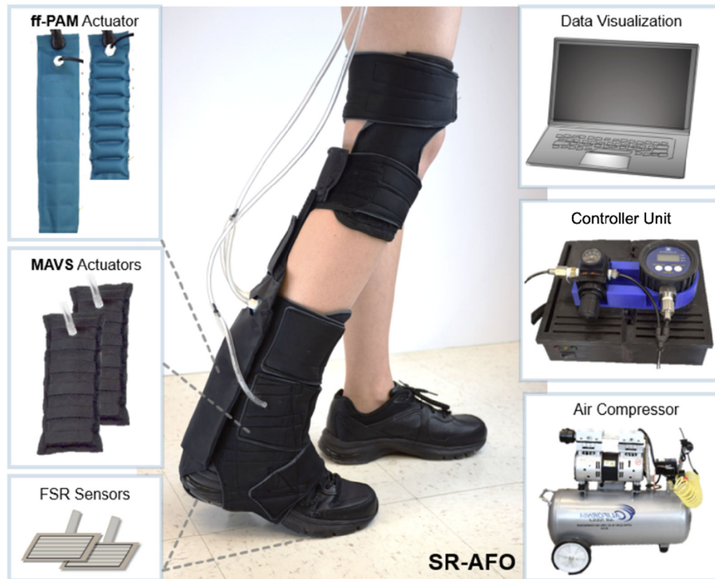
Figure 11. (Middle) The final assembly of the SR-AFO and its components. (Left) The ff-PAM and MAVS actuators and the FSR sensors for gait detection. (Right) The controller, pneumatic source (air compressor), and visual feedback for system operation.
