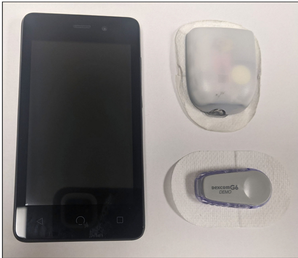
Figure 4. Omnipod patch pump ( top right ) with personal diabetes manager ( left ) and Dexcom G6 continuous glucose monitor ( bottom right ).
