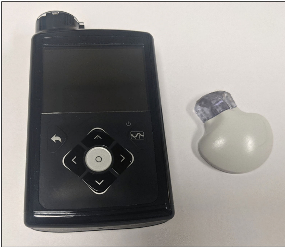
Figure 1. Medtronic 670G insulin pump ( left ) with Guardian Sensor 3 continuous glucose monitor ( right ).
