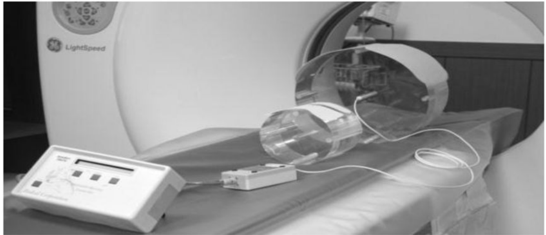
Figure 4. Ionization chamber, PMMA phantom and bismuth shielding for CT dose measurement.
