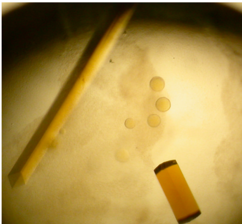
Figure 2. Crystals of unsubstituted recombinant HADH grown in 0.1 M HEPES buffer (pH 7.4) containing 2.0 M (\text{NH}_4)_2\text{SO}_4 , 2% 400-PEG (v/v), and 4% glycerol (v/v). Crystal to the left is a square rod like those used to collect data, while the crystal on the rod is one of the square “pizza box” crystals viewed edge-on.
