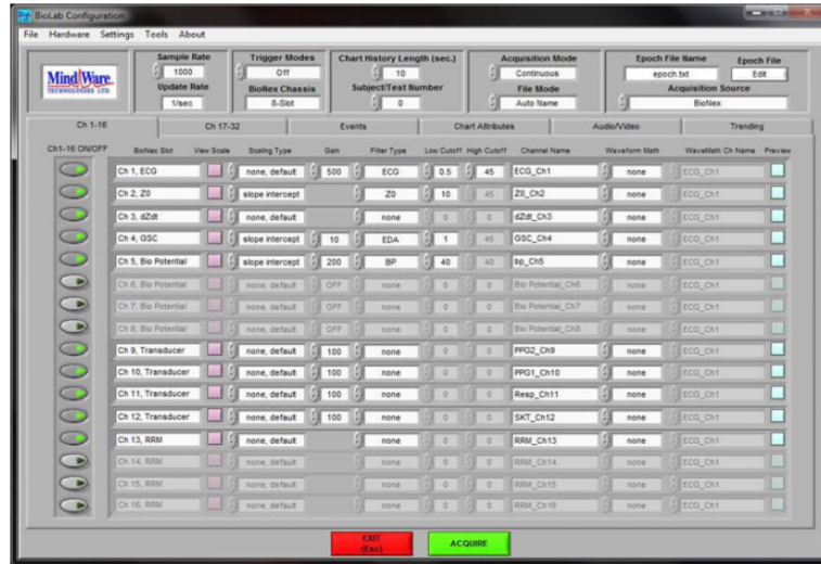
Figure 1. BioLab Software Configuration settings This figure displays a screenshot of the configuration settings to be used during ANS data collection as described in step 1.2.
