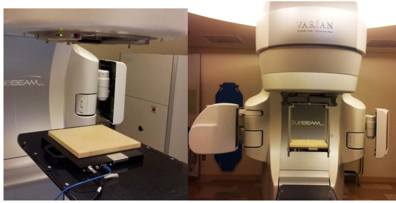
FIG. 1. The (a) on-couch stationary and (b) on-head rotational settings for the EPID system.
