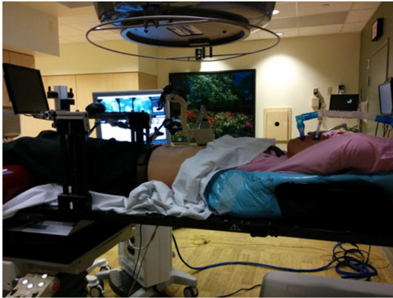
Fig. 3. Volunteer setup in the treatment room with ultrasound system and ABC. The gantry rotated around the volunteer to assess clearance.
