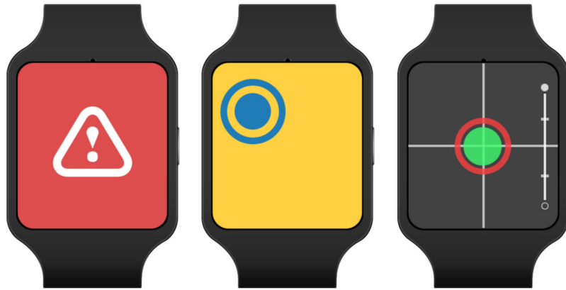
Fig. 1. Modes indicating different states (from left to right): tool outside of tracking range, tool far away from insertion point, tool in close enough distance to insertion point.
